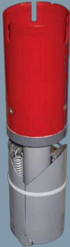
Inclinometer Casing Anchor prior to arm extension.
