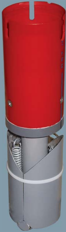
Inclinometer Casing Anchor prior to arm extension.
