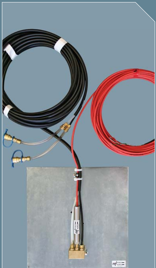
Typical installation of a Vibrating Wire Liquid Settlement System.
