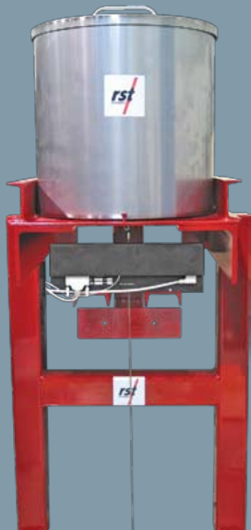
Inverted Pendulum shown with RxTx Telependulum.
