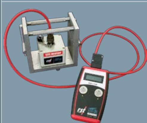
Portable Tilt meter shown with the IC6800S Readout
