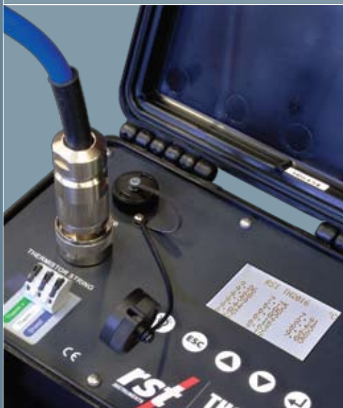
Thermistor string connector attached to the TH2016 Thermistor Readout.
