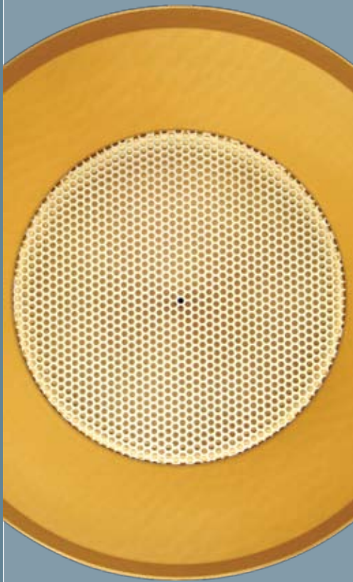
Aerial view of Tipping Bucket Rain Gauge showing filter screen and funnel.
