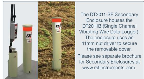
The DT2011-SE Secondary Enclosure houses the DT2011B (Single Channel Vibrating Wire Data Logger). The enclosure uses an 11mm nut driver to secure the removable cover. Please see separate brochure for Secondary Enclosures at [www.rstinstruments.com](http://www.rstinstruments.com).
