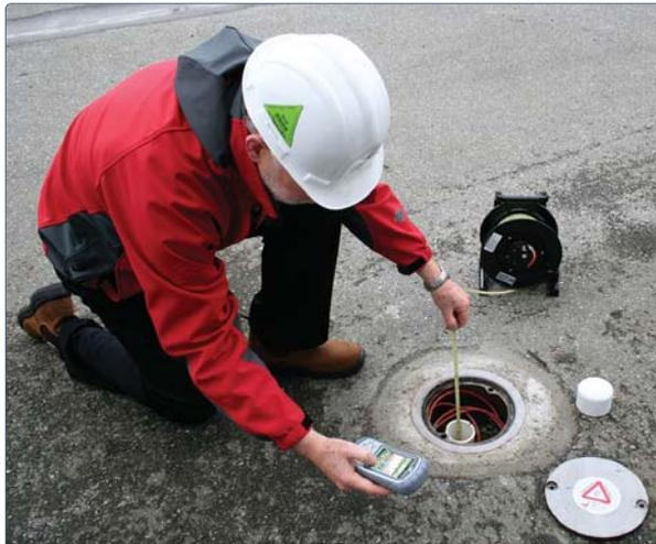
Water level readings being manually entered into FieldBook Software at a project site.
