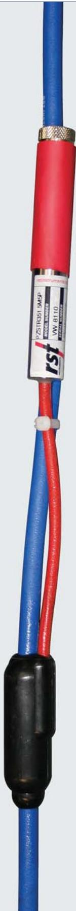
Traditionally, multiple piezometer installations in a borehole was slow, complex, and subject to unintended communication between piezometers. Grouted piezometers are quick and easy to install, have excellent zone isolation, and have rapid response to pore pressure changes. The fully grouted method is increasingly the preferred standard approach for installing piezometers in boreholes. For more information see:
