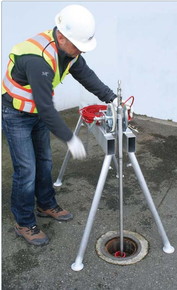
The HOSS shown with an attached Vertical In-place Inclinerometer being lowered into a borehole with installed inclinometer casing.
