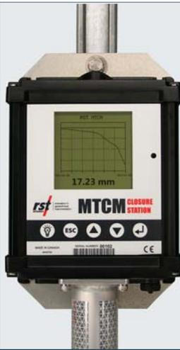
The large graphics display has a convenient backlight and can be activated by pushing any button.
