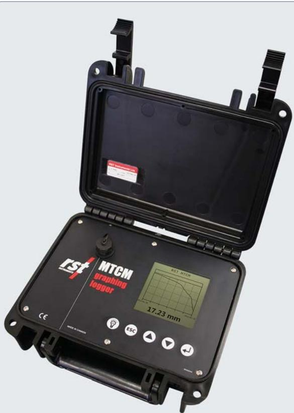
The MTCM - Graphing Logger is a rugged and compact unit that is also light-weight and can be easily carried in one hand.
