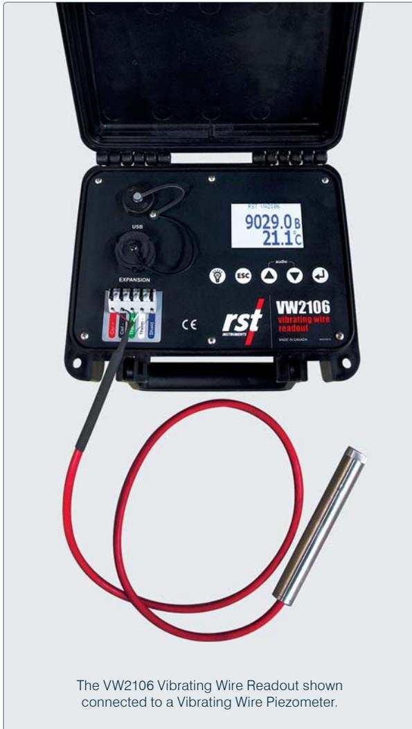
The VW2106 Vibrating Wire Readout shown connected to a Vibrating Wire Piezometer.
