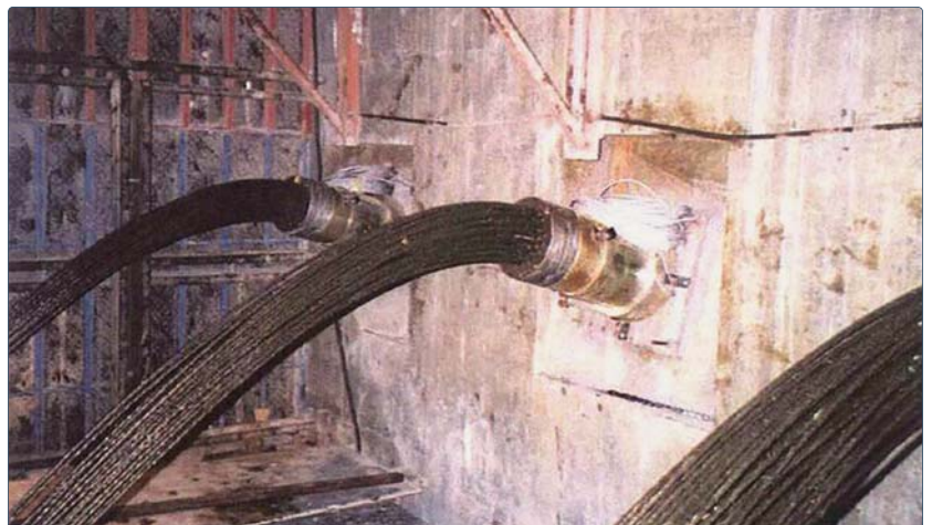
High capacity load cells for multi-strand anchors used in the seismic retrofit of a dam.
