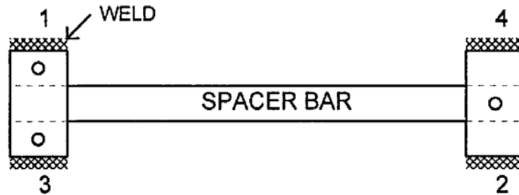
FIGURE 3-3 WELDING SEQUENCE FOR THE MOUNTING BLOCKS
