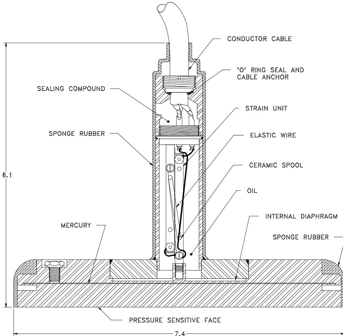
The interface stress meter is so called because it is adapted to the measurement of compressive stress against a surface. It is similar to the concrete stress meter, but it has much thicker plates to make it independent of the distribution of force against it.
