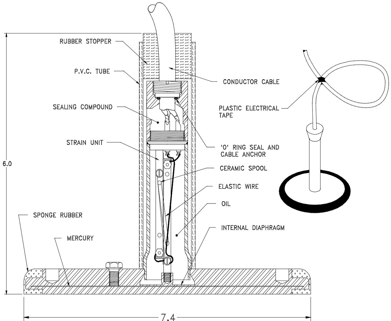
The concrete stress meter is a 7.3 - inch diameter plate with a strain-meter sensing element mounted on one face. The plate has a mercury film at its mid-thickness and a flexible rim with the result that any stress through the plate is applied to the mercury film. Extraneous deformations such as those due to drying shrinkage, have very little effect on stress through the plate (and the mercury) so the calibration is in terms of compressive stress per
