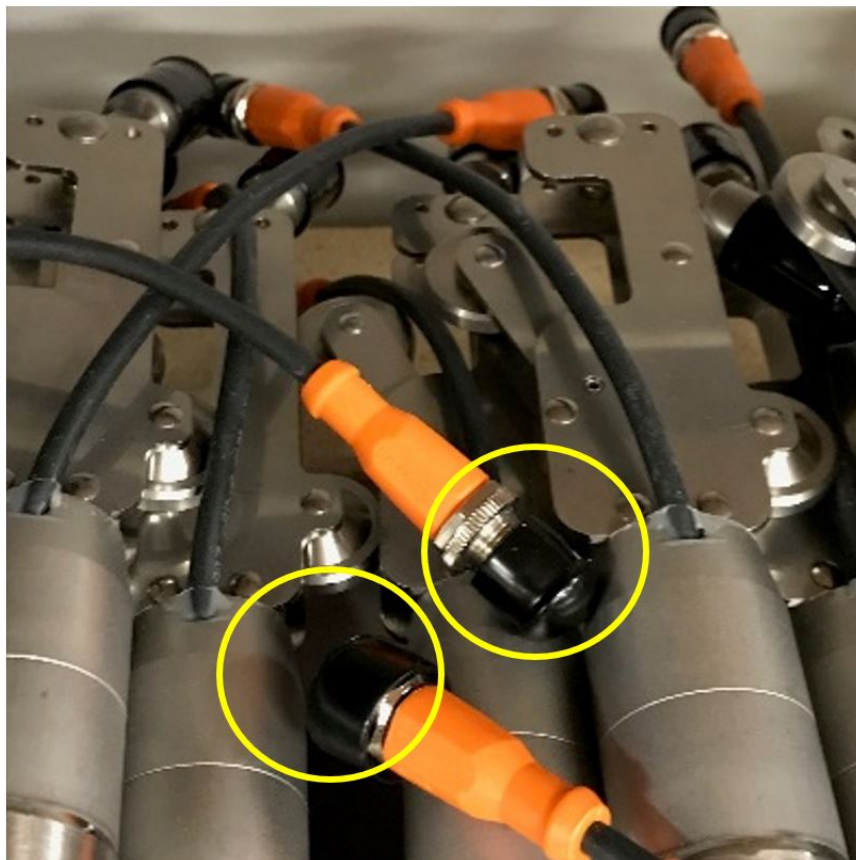
Figure 6: Ensure Protective Caps are Always on the Connectors
