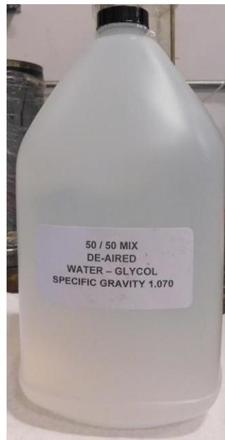
**FIGURE 3-1 50% BY VOLUME GLYCOL AND WATER SOLUTION**
