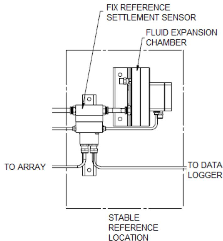
FIGURE 5-1 REFERENCE SENSOR AND CONNECTION TO DATA LOGGER
