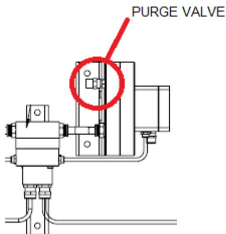
**FIGURE 4-5 PURGE VALVE ON REFERENCE SENSOR**
