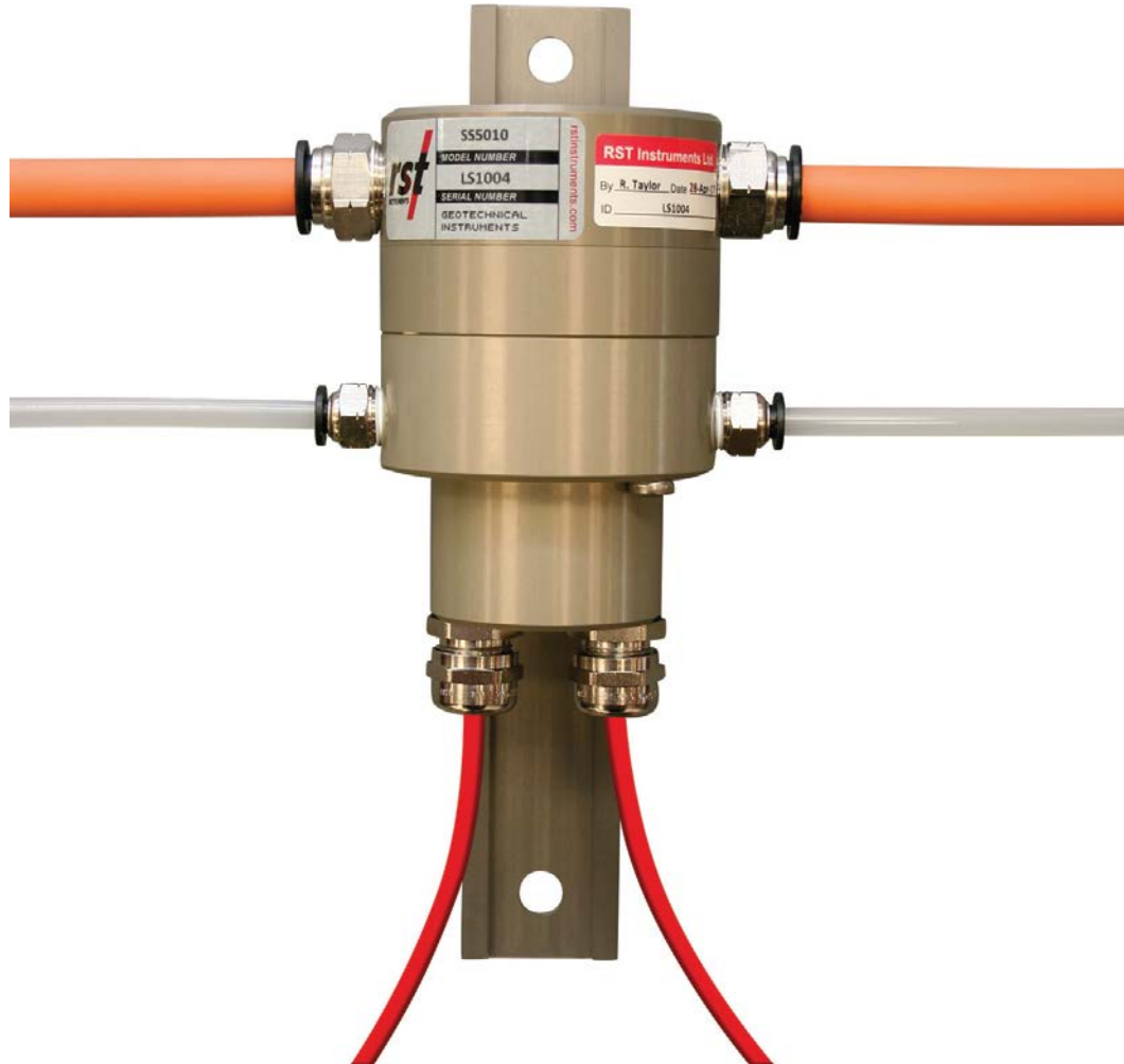
FIGURE 4-1 PRECISION LIQUID SETTLEMENT SENSOR
