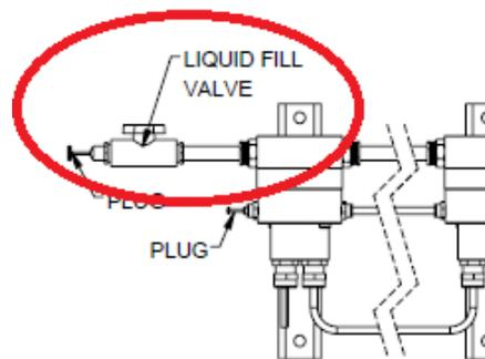
**FIGURE 4-4 LIQUID FILL VALVE**
