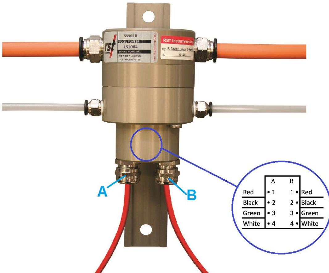
**FIGURE 4-2 SENSORS AND CABLE GLANDS**
