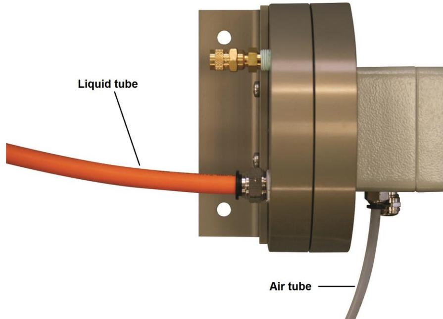
**FIGURE 4-3 PRECISION LIQUID SETTLEMENT FLUID EXPANSION CHAMBER, WITH LIQUID TUBE AND AIR TUBE**
