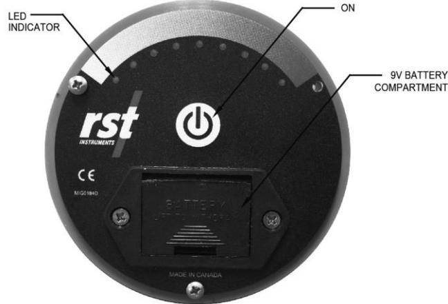
Figure 3: Reed Switch Probe Controls
