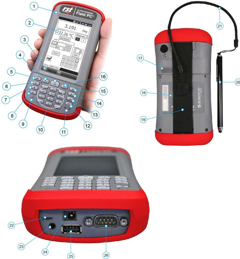
**Figure 2: Overview of the Ultra-Rugged Field PC<sup>2</sup><sup>TM</sup>**
