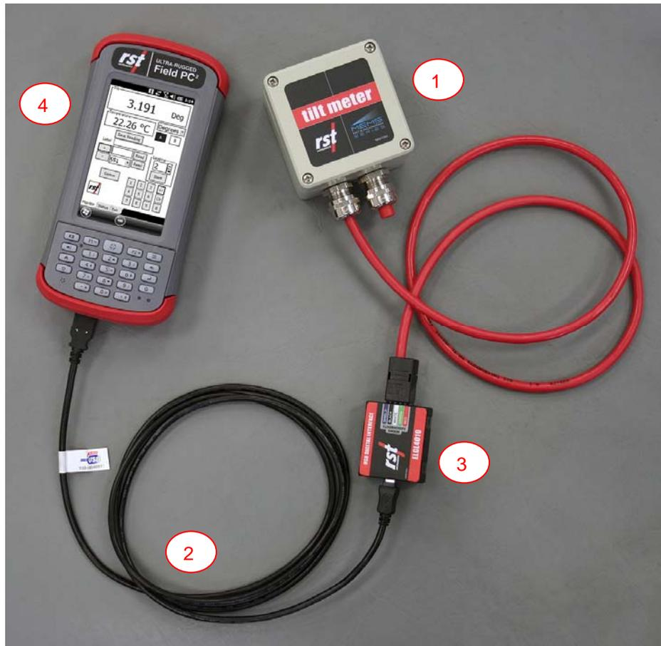
**Figure 4 – Digital Tilt Bus System Overview**
