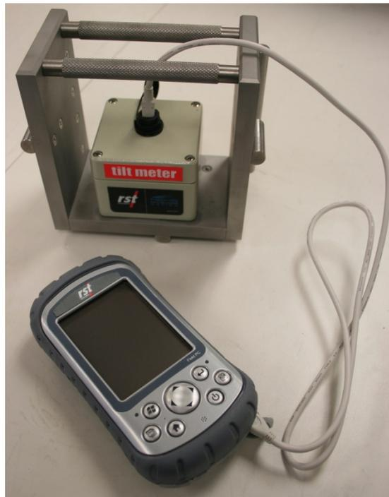
**Figure 1: MEMS Portable Tiltmeter & MEMS Portable Tiltmeter Readout**
