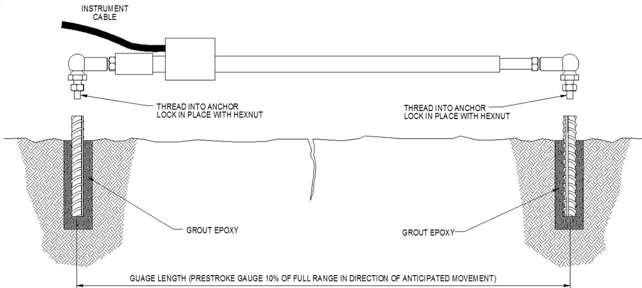
**Figure 3: Installing Crackmeter**
