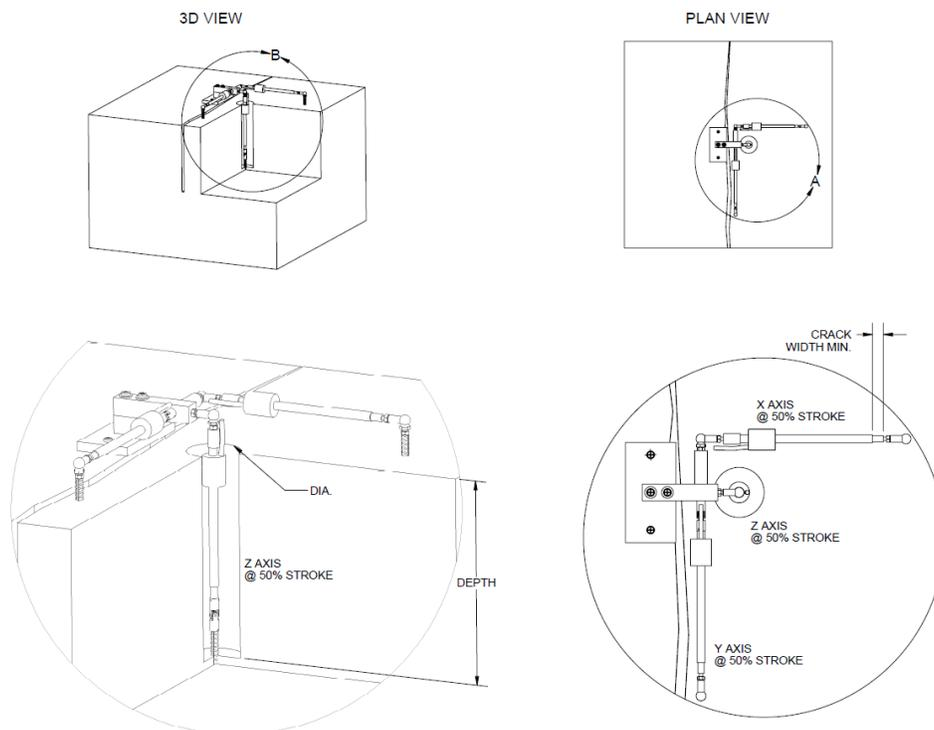
**Figure 4: Submersible 3D VW Crackmeter General Arrangement**
