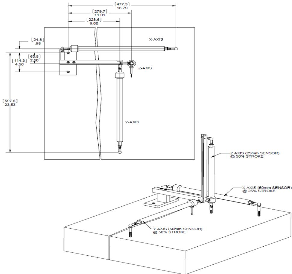
Figure 7: Submersible 3D VW Crackmeter General Arrangement
