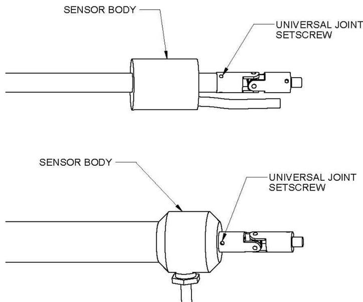
**Figure 5: Installing the Y-axis on a 3D Crackmeter**
