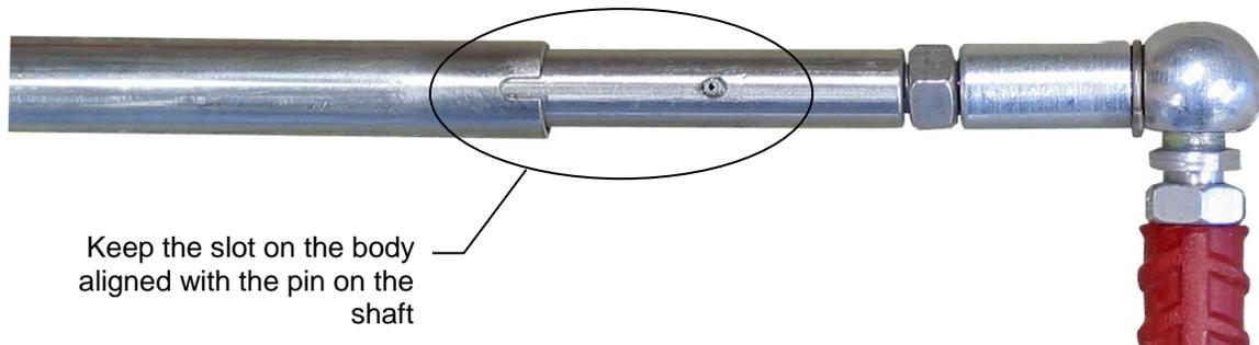
**Figure 2: Instrument Shaft Alignment**
